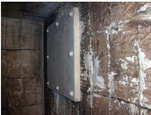
**Fig. 5. Photo showing a board bolted to a target wall**
